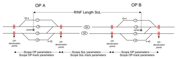
Fig. 3 – Section of Line (SoL) between two Operational Points (OP) (provided by D. KES)
